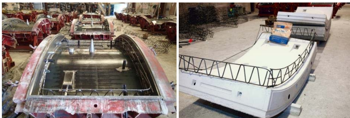
Figure 6: Segment mould with bursting ladder in place (left) and a cast segment with BarChip macro synthetic fibre as primary reinforcement and (provisional) bursting ladder as secondary reinforcement (right)
