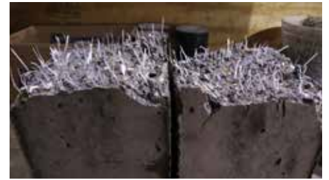
Image 5: QC Testing of BarChip fibre reinforced segments.
