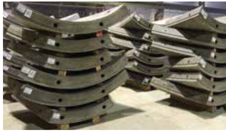
Image 4: Post-production stacking of BarChip fibre reinforced segments.
