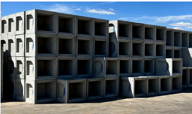
Stormwater Pits: Removed steel mesh, eliminating 1 whole day of prep work in 2-day the production cycle.
