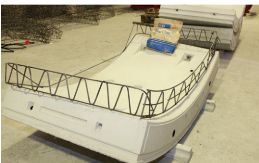
Santona Laredo Tunnel: Switching from steel cage to BarChip reduced total segment costs by nearly 40%.
