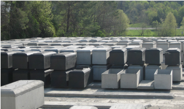
Burial Vaults: Eliminated steel reinforcement from vaults and lids, reducing costs and increasing production speeds.
