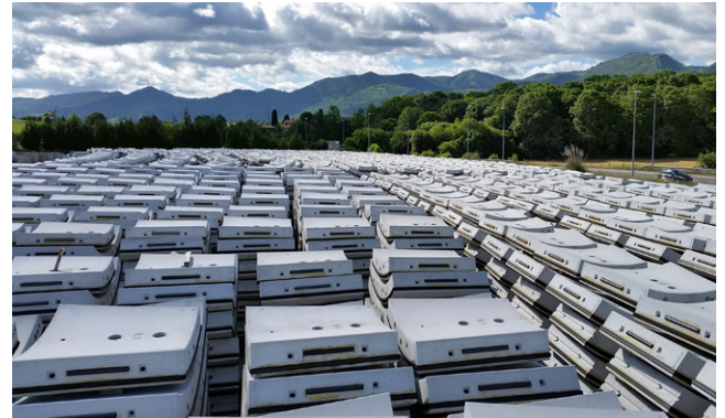
Santona Laredo Tunnel: BarChip reduced carbon footprint by 77% from original steel design & overall segment costs by ~40%
