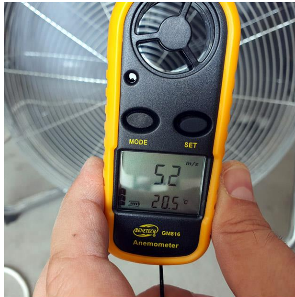
Figure 6. Measuring the wind speed with an anemometer
