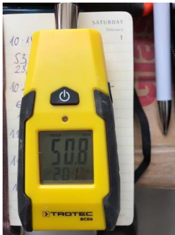
Figure 10. Measuring of the temperature and humidity in the tent during the test (the climate control device was inside of the testing tunnel, and taken out for photograph)
