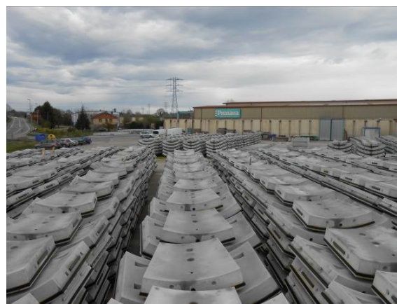
Figure 22. Segment storage in the precast plant
