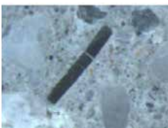
Image 3: Poor quality synthetic fibres can suffer from mechanical failure and damage such as fissioning (top) and splitting (bottom) during shotcreting operations (Kaufmann 2014).
