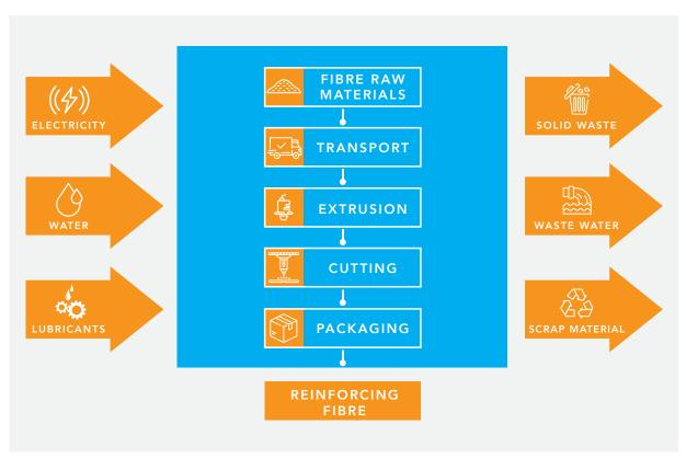
Figure 1: Flow diagram of production system
