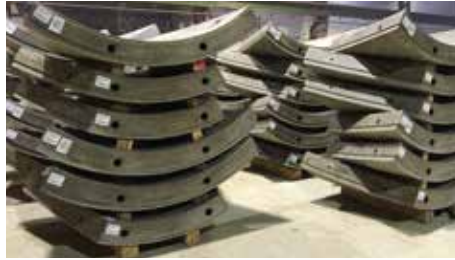
Image 3: Post-production stacking of BarChip fibre segments.
