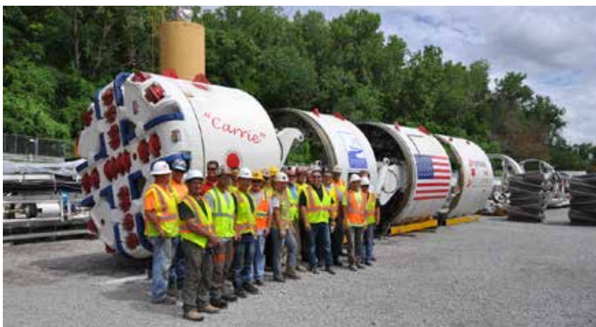
Image 2: Blacksnake EPB Tunnel Boring Machine
