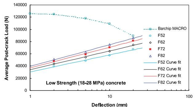
In low strength concrete (18 -28 MPa), BarChip Macro dosed at 3 kg/m<sup>3</sup> outperforms traditional steel reinforcement up to 20 mm deflection. A 12 mm deflection is roughly equivalent to a 5 mm crack width.
