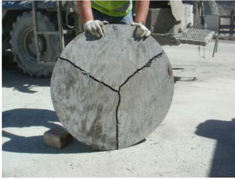
Figure 3. Panel displaying the characteristic crack pattern [12]
