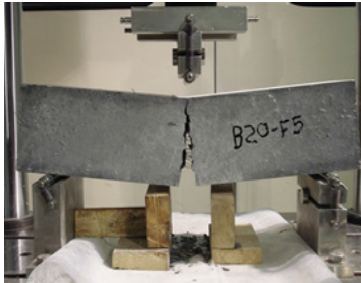
Figure 2-2: Crack bridging by fibres in a beam test
