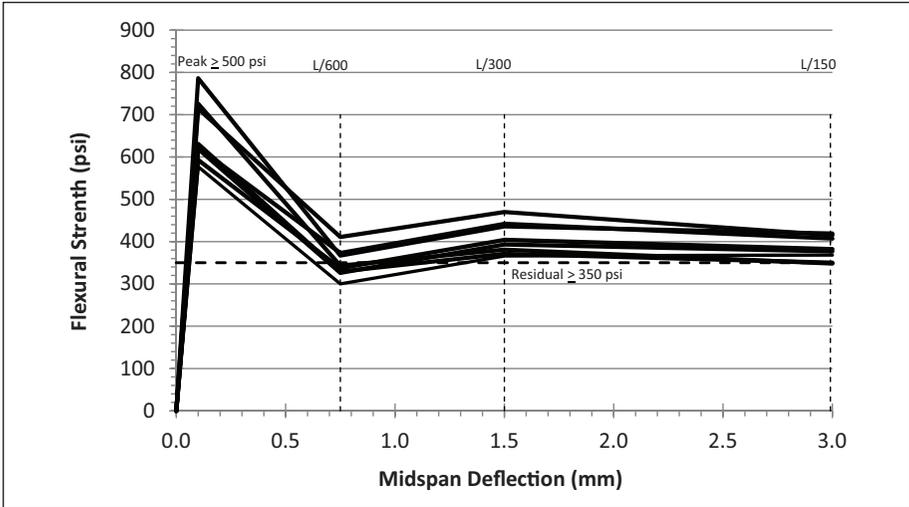
**Figure 4. Flexural strength results for tests performed during tail and starter tunnel pours (ASTM C1609)**
