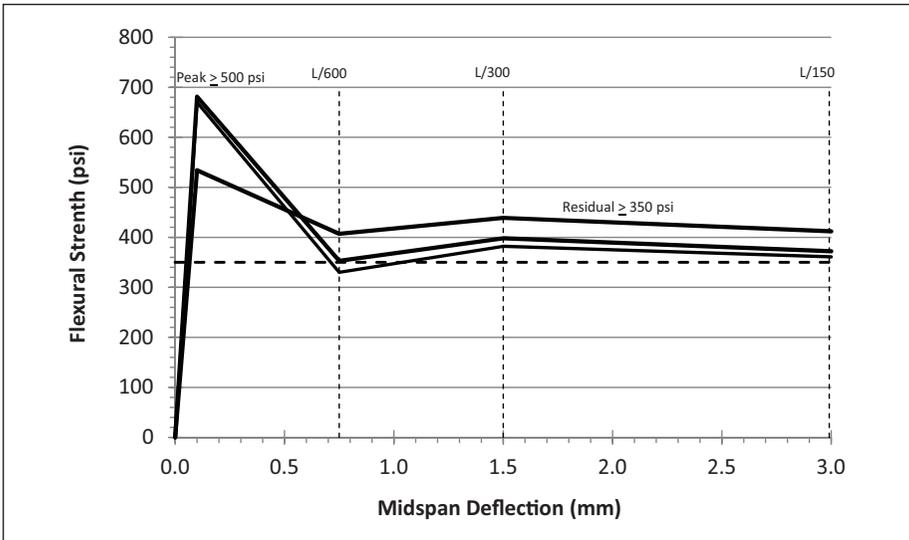
Figure 2. Flexural strength results for trial batches (ASTM C1609)
