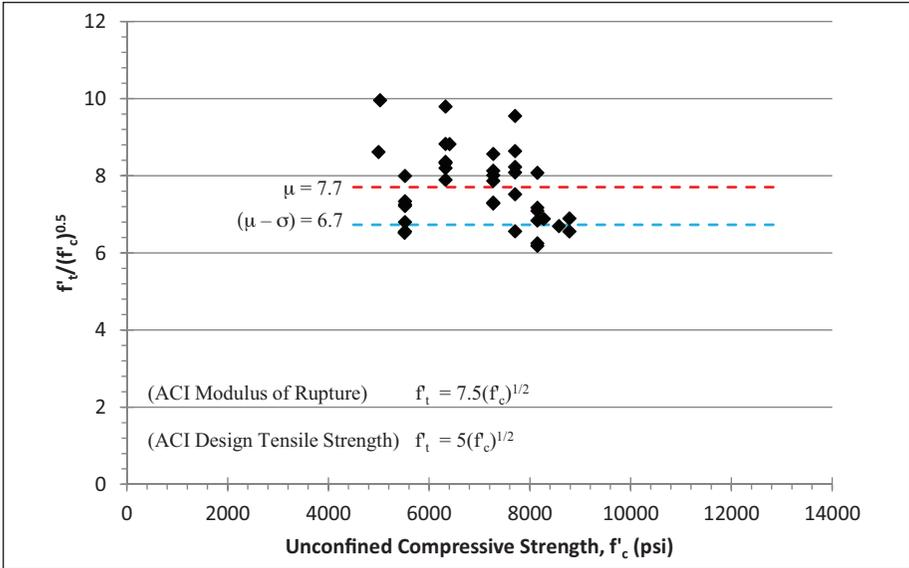
Figure 5. Normalized flexural strength results for tests performed during tail and starter tunnel pours (ASTM C1609).
