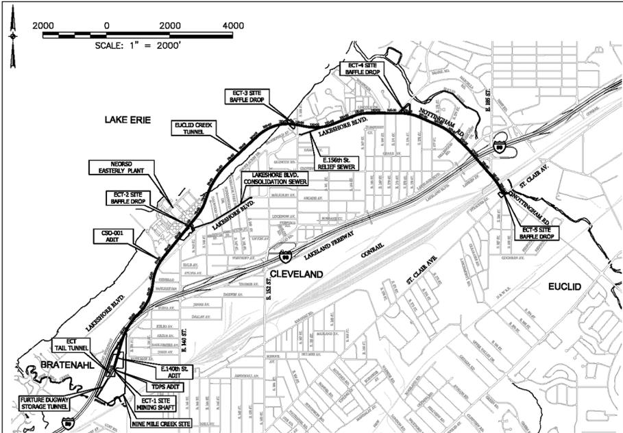
Figure 1. Euclid Creek Tunnel project layout
