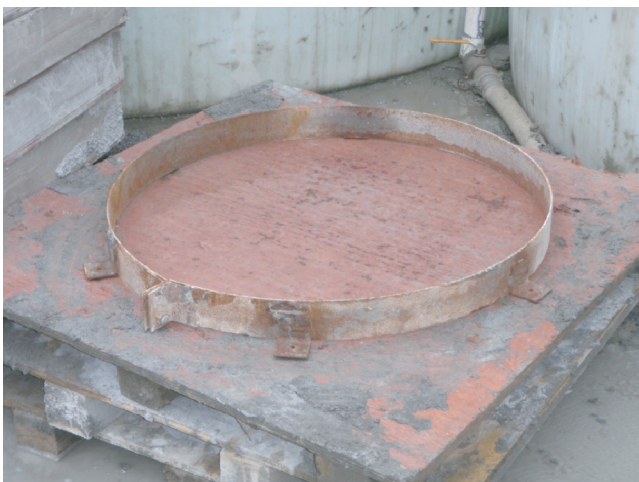
FIGURE 5 Metal form for panels mounted on wooden pallet.
