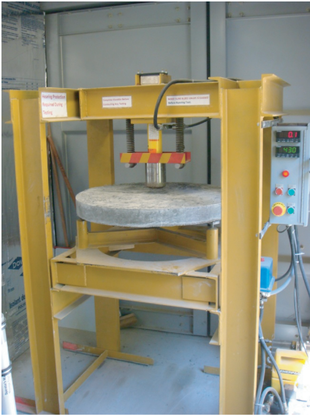
FIGURE 4 RDP test machine with panel.
